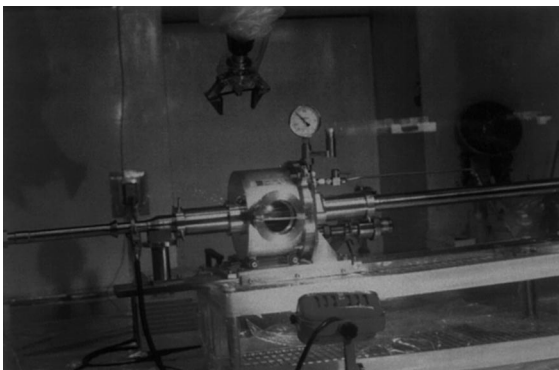
Fig. 4. Remote control welding work in the hot cell.
